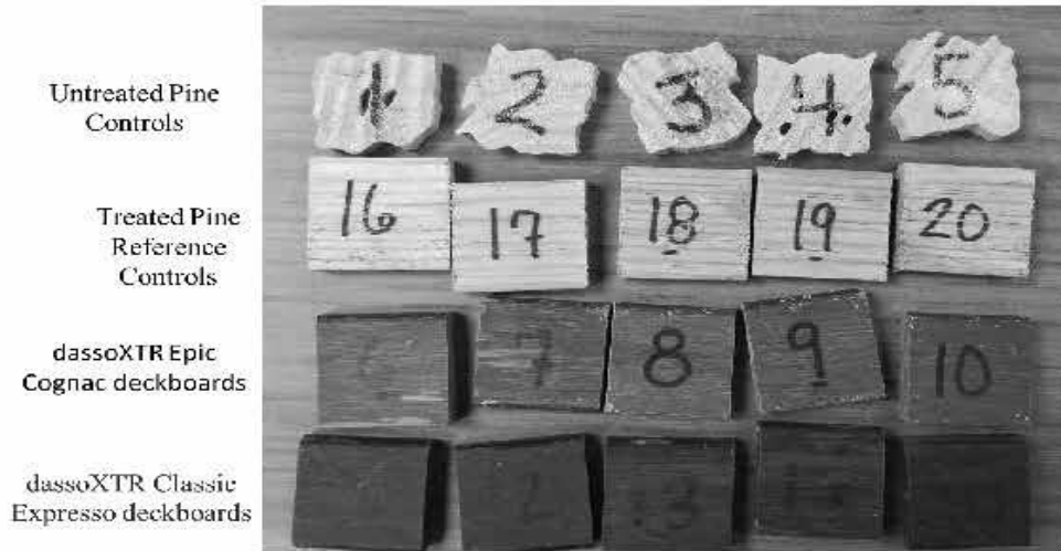
Figure 2. Test samples including controls and deckboards
